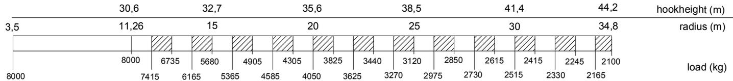
**LIFTING CHART Outrigger spread 6,90 m x 5,15 m**
